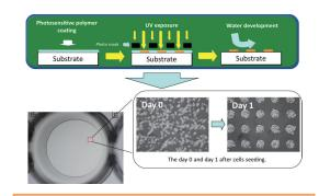
Photolithographic process to fabricate 3-dimensional cell structure: Chemical surface modification using photosensitive & non cell-attaching polymer on the cell culture plate
